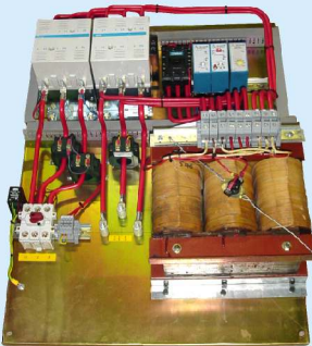
AUTO TRANSFORMER STARTER
